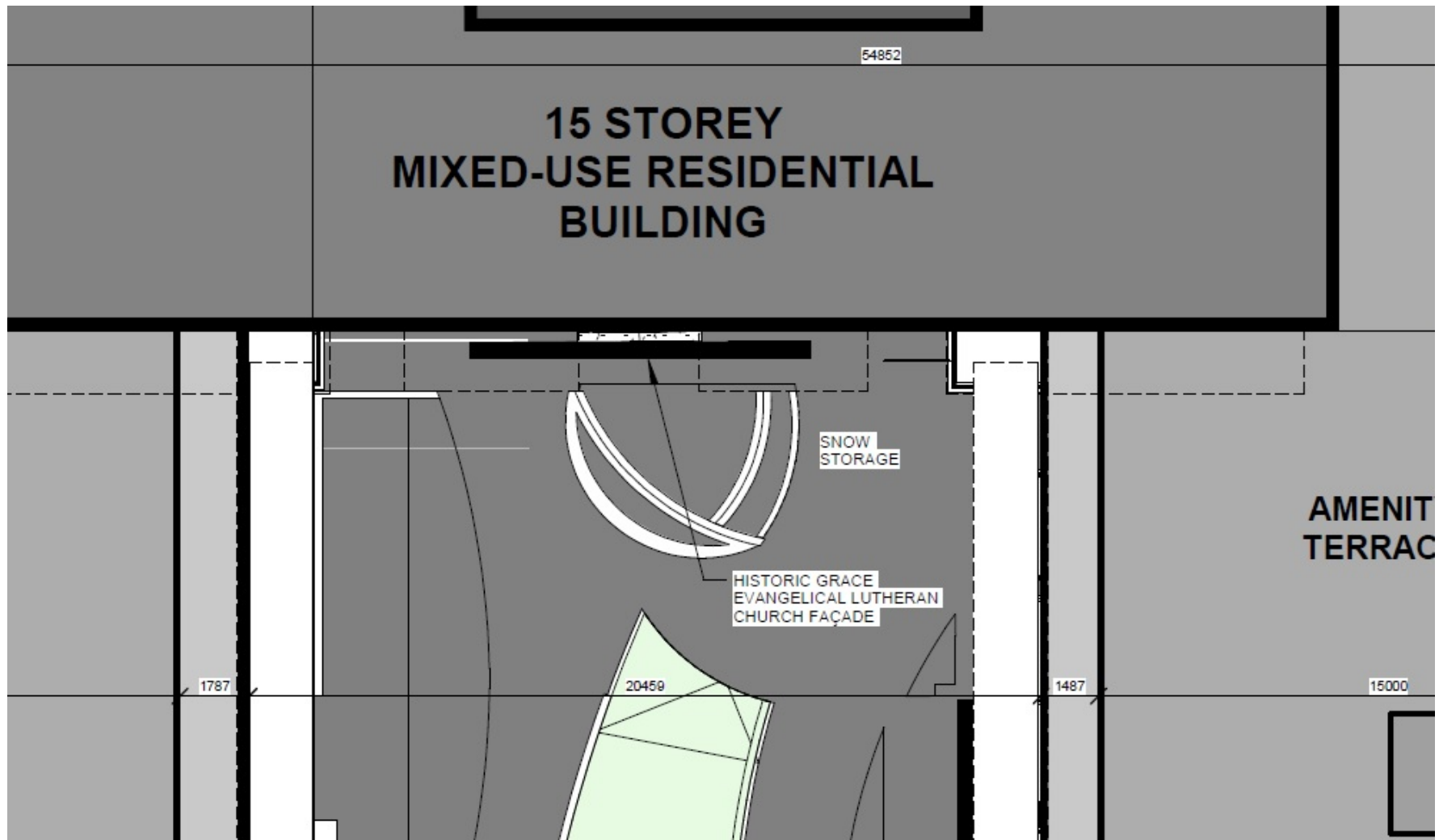
Architectural Drawings 20: The church façade will be rebuilt and integrated into the courtyard to act as a passthrough from the semi-public outdoor courtyard to the more private covered outdoor space.
